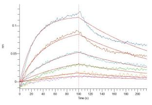
Loaded Human VEGF Antibody (5E7)-Fc on AHC Biosensor, can bind Mouse VEGF164(Cat#MA0616) with an affinity constant of 3.63 nM as determined in BLI assay.
